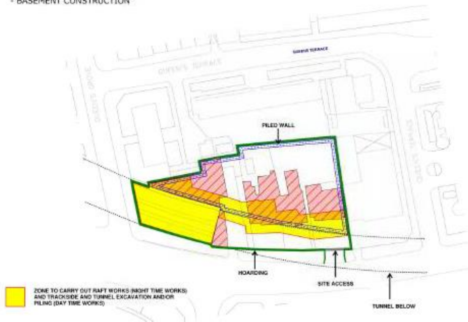
Figure 3 – Demolition and Construction Sequence Stages 1 & 2
